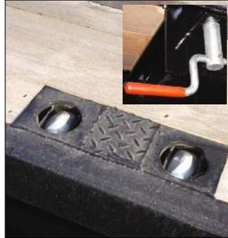
The platform skeletal is supplied with recessed twistlocks and doubles as either a skeletal to handle the full range of ISO containers or as a flat platform.
