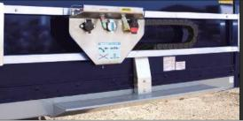
Developed to aid safety, MAVIS (Montracon articulated vehicle interconnecting system) can be slid to either side of the trailer to facilitate un/coupling and eliminating the need for the driver to climb onto the chassis between the cab and trailer.
