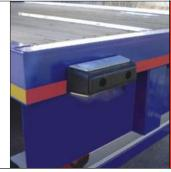
The option of sockets and stanchions extends the load versatility of the flat to include the movement of all from logs to oil field drilling equipment. Stanchions are neatly stowed beneath the frame or on the headboard for flat platform operation.
