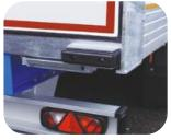
Carefully positioned reinforced buffers minimise the risk of damage when reversing up to a loading bay, for example.
