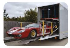
Designed to accommodate racing cars and crew, yet be low enough to access the pits via tunnels under the race track.
