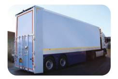
Rear door/tail lift arrangement designed to meet retail delivery requirement.
