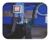
To ease loading/unloading, the trailer deck is easily raised or lowered at the rear to match dock height. An automatic trip restores the deck to normal running height on departure.
