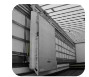
Internally installed lift, with fore/aft movement to ease loading and unloading capability.
