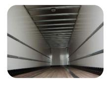
A 'high gloss' finish inside and out helps to maintain a clean, neat appearance, with an ample kick strip providing scuff protection during loading/unloading. Load restraining rails are side panel mounted.
